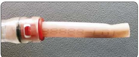
*In this case, the technician had mounted a cable tip with half a millimetre larger diameter than the fiber cable. The tip became fully wedged in the bend.*
